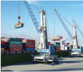
Mobile Harbour Crane
