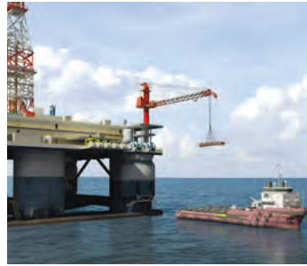
Offshore Pedestal Crane
