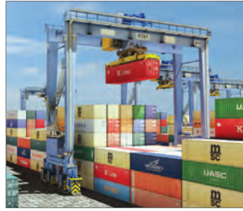
Rubber Tyred Gantry Crane
